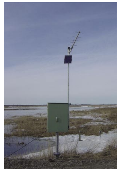
Hydrometric gauging station along Medora Creek.
