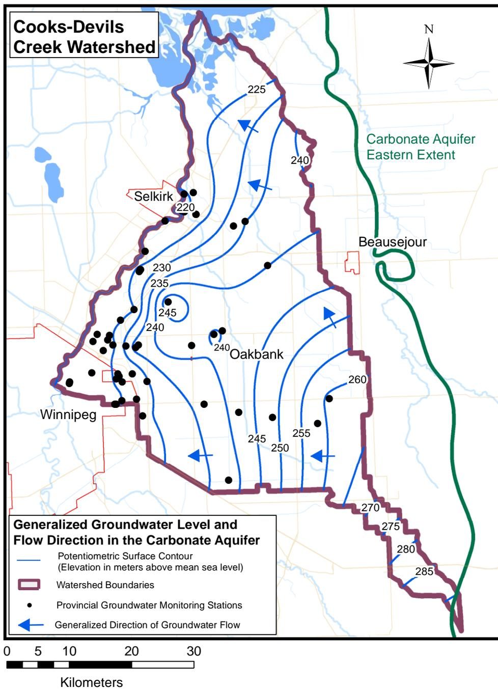
**Map # 7 – Location of Provincial Groundwater Monitoring Wells Completed in the Carbonate Aquifer and Generalized Groundwater Flow Direction**
