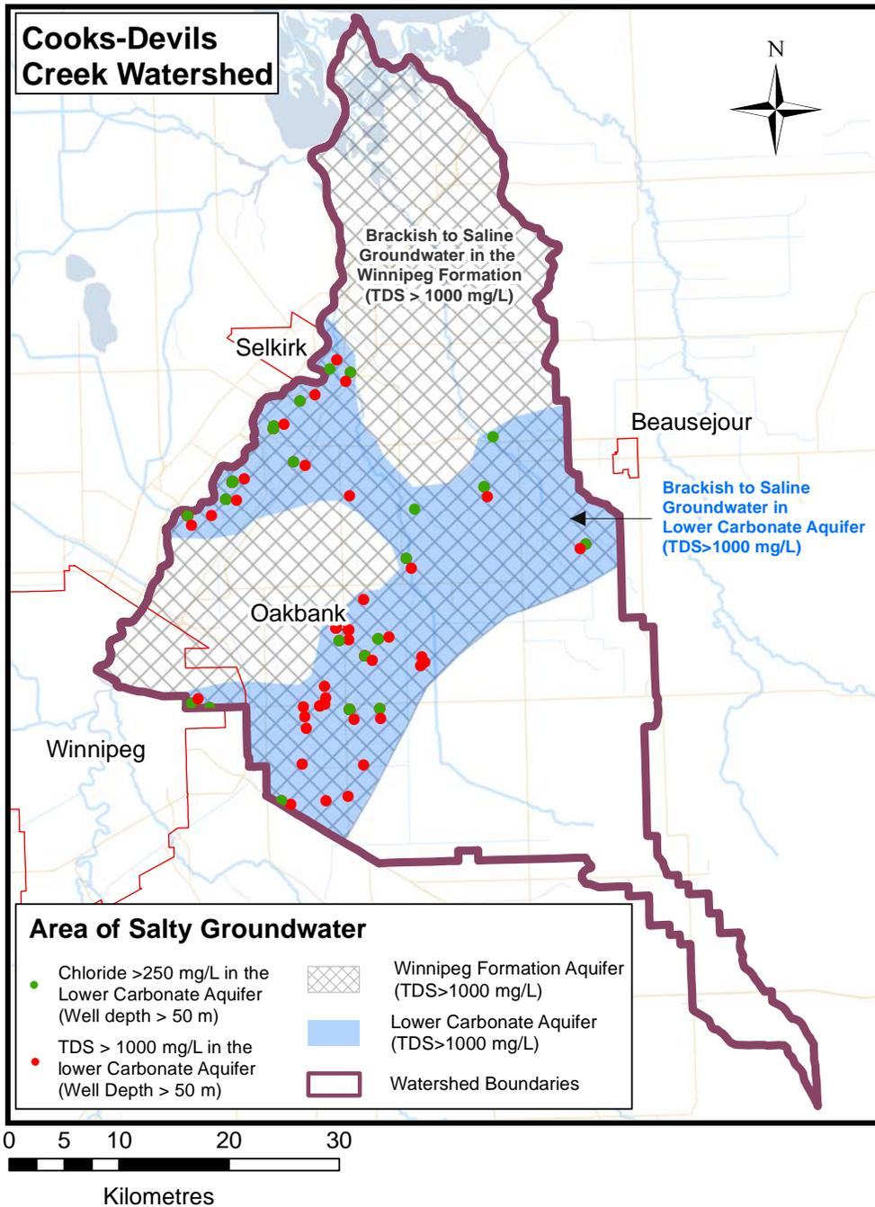
**Map # 8 – Area of high total dissolved solids in the Winnipeg Sandstone Aquifer and in the Lower Carbonate Aquifer**
