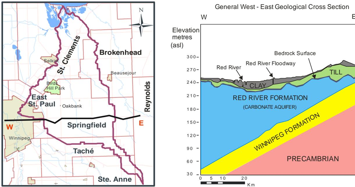
Figure 2. Aquifer Geology Map and Cross Section (Source: Groundwater Availability Study, Winnipeg Area 1974)
