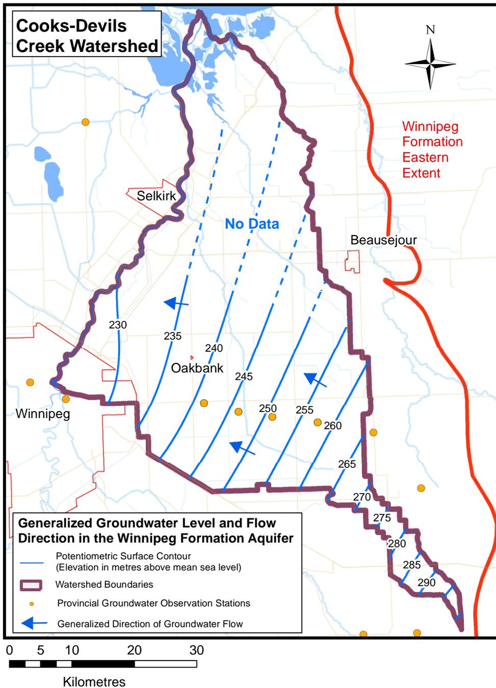
**Map # 6 – Location of Provincial Groundwater Monitoring Wells Completed in the Winnipeg Sandstone Aquifer and Generalized Groundwater Flow Direction**
