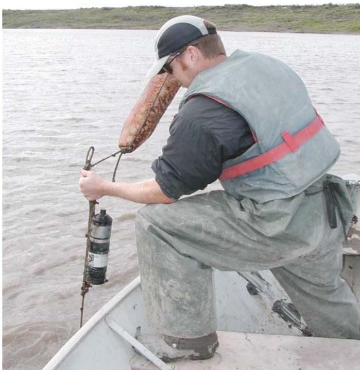
Figure 9. Deployment of a stationary receiver, showing steel cable, receiver, and float.
