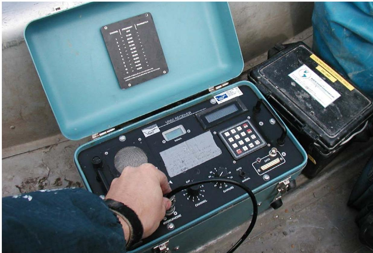
Figure 13. VR-60 acoustic receiver used for manual tracking of fish at the Kelsey GS, June-September, 2006.
