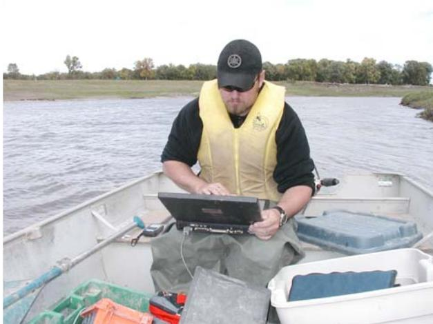
Figure 10. Downloading acoustic data from a stationary receiver onto a PC.
