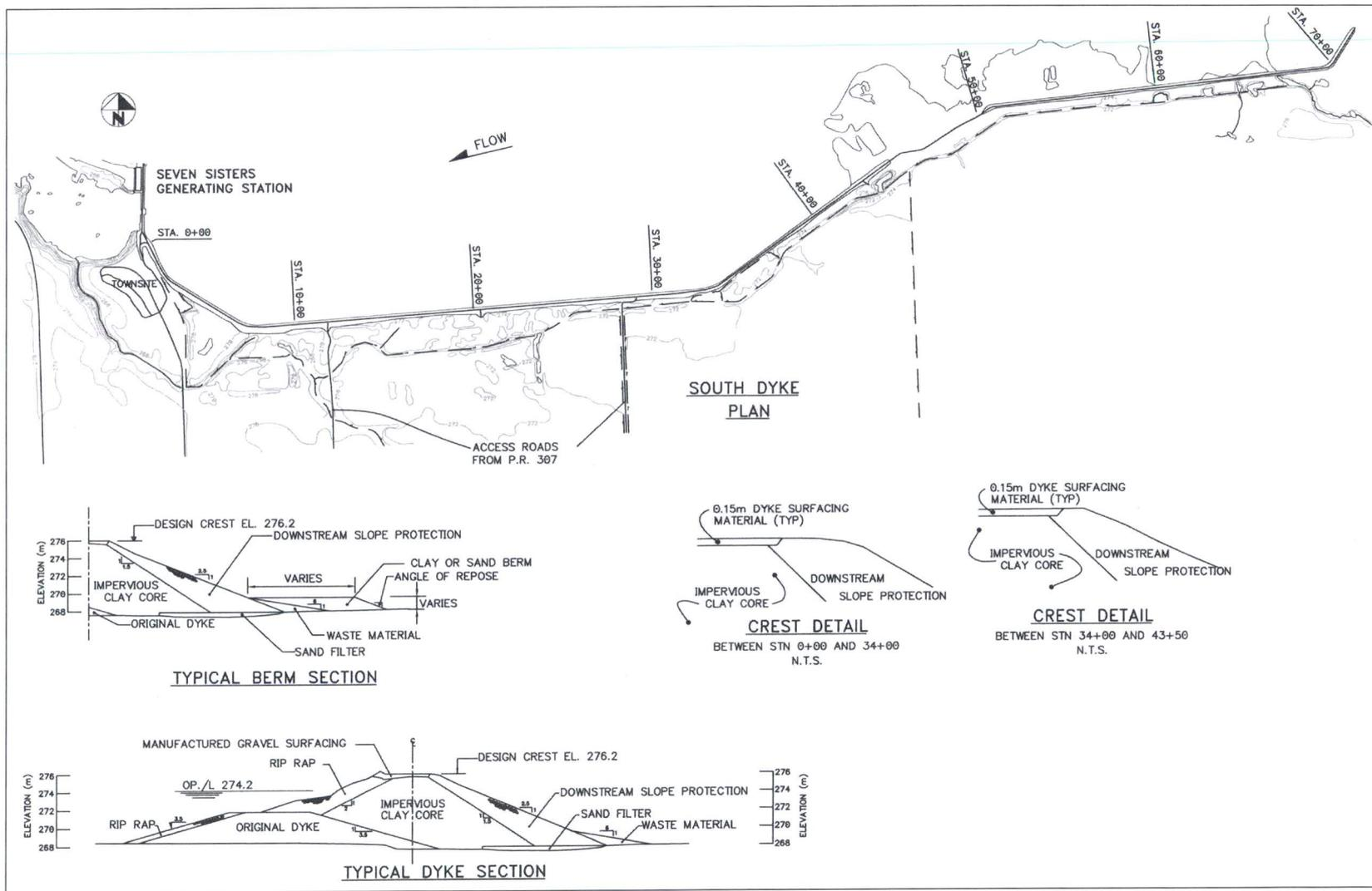
Figure 5: South Dyke - Plan and Typical Sections
