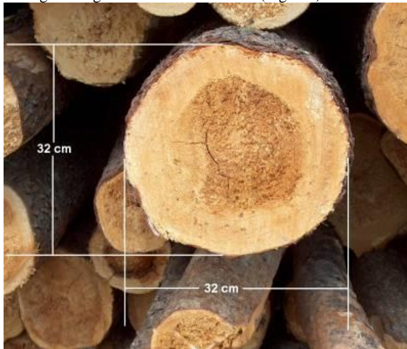
Figure 2 Measuring diameters: logs with regular sawn surfaces
