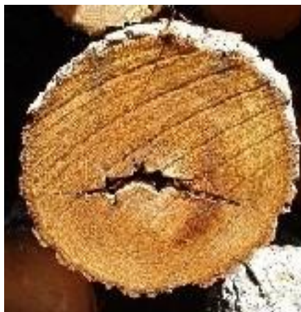
Figure 23 Heart check on the end surface of a log
