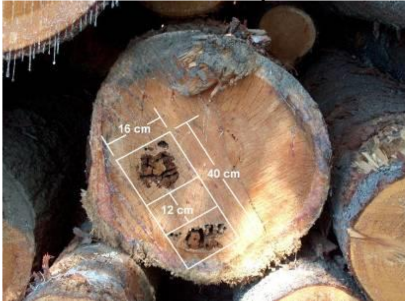
Figure 24 Two defects separated by 14 cm or less
