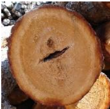
Figure 23 Heart check on the end surface of a log
