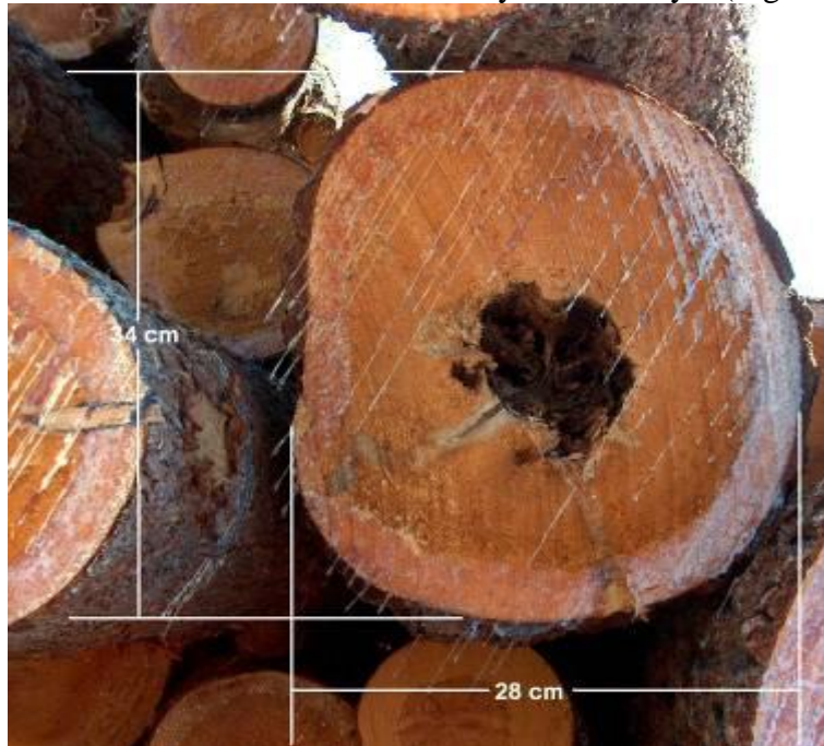
Figure 3 Measuring diameters: logs with irregular sawn surfaces
