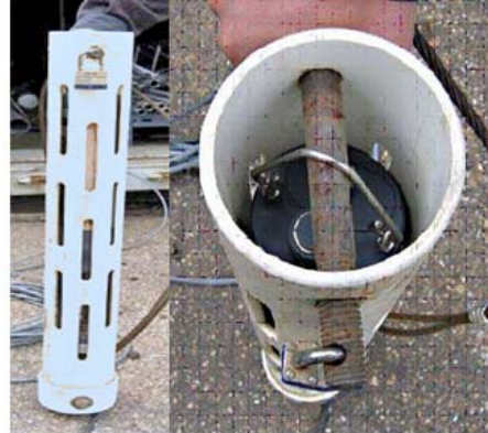
Photo 9 Left. A sonde with a number of probes and a wiper (Source: B.C. B.C. Ministry of Environment (2006))
