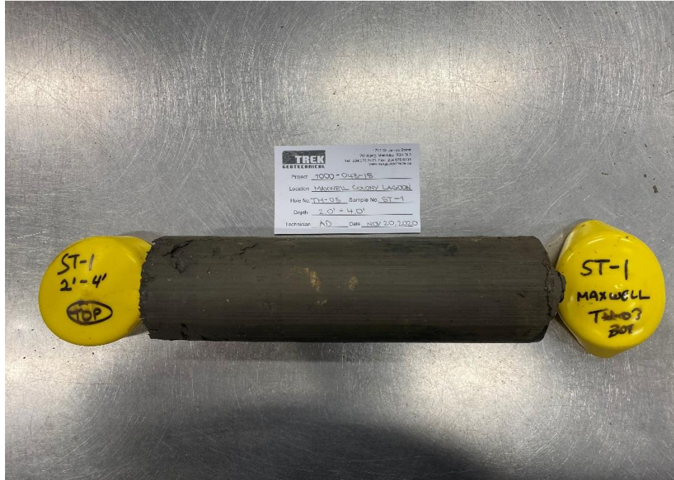
Photo 1: Extruded Shelby Tube at Test Hole TH-03_ST-1
