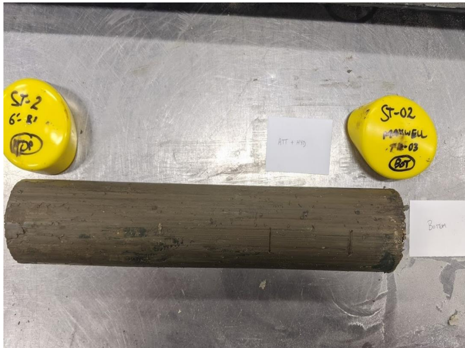
Photo 2: Extruded Shelby Tube at Test Hole TH-03_ST-2
