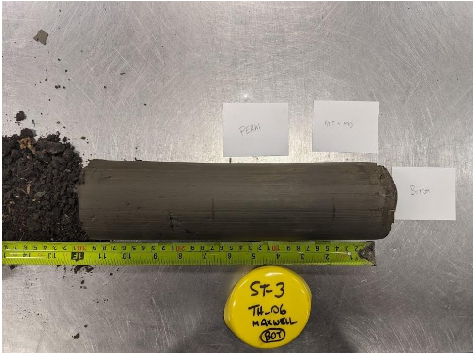
Photo 3: Extruded Shelby Tube at Test Hole TH-06_ST-3
