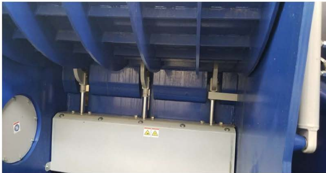
The screen locks "Locked Position"
