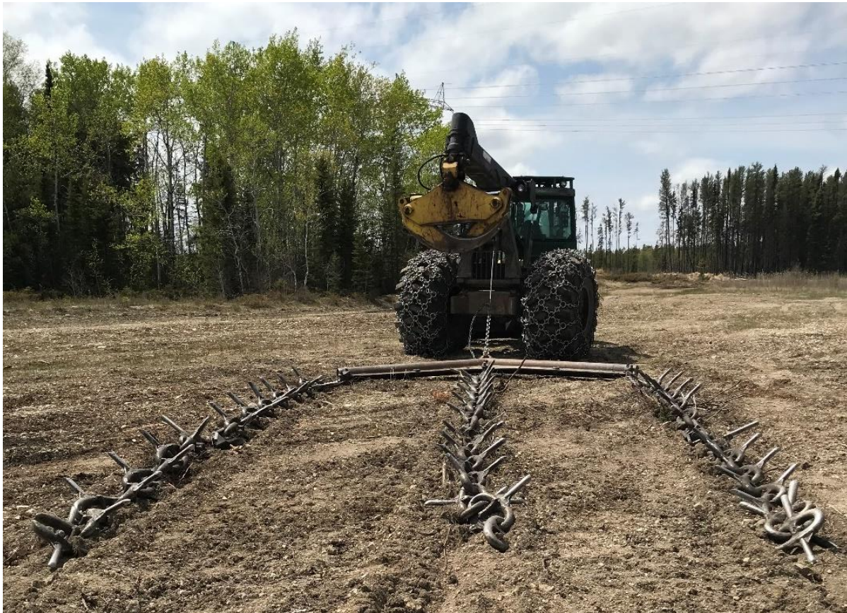
Spiked anchor chains used for scarification.
