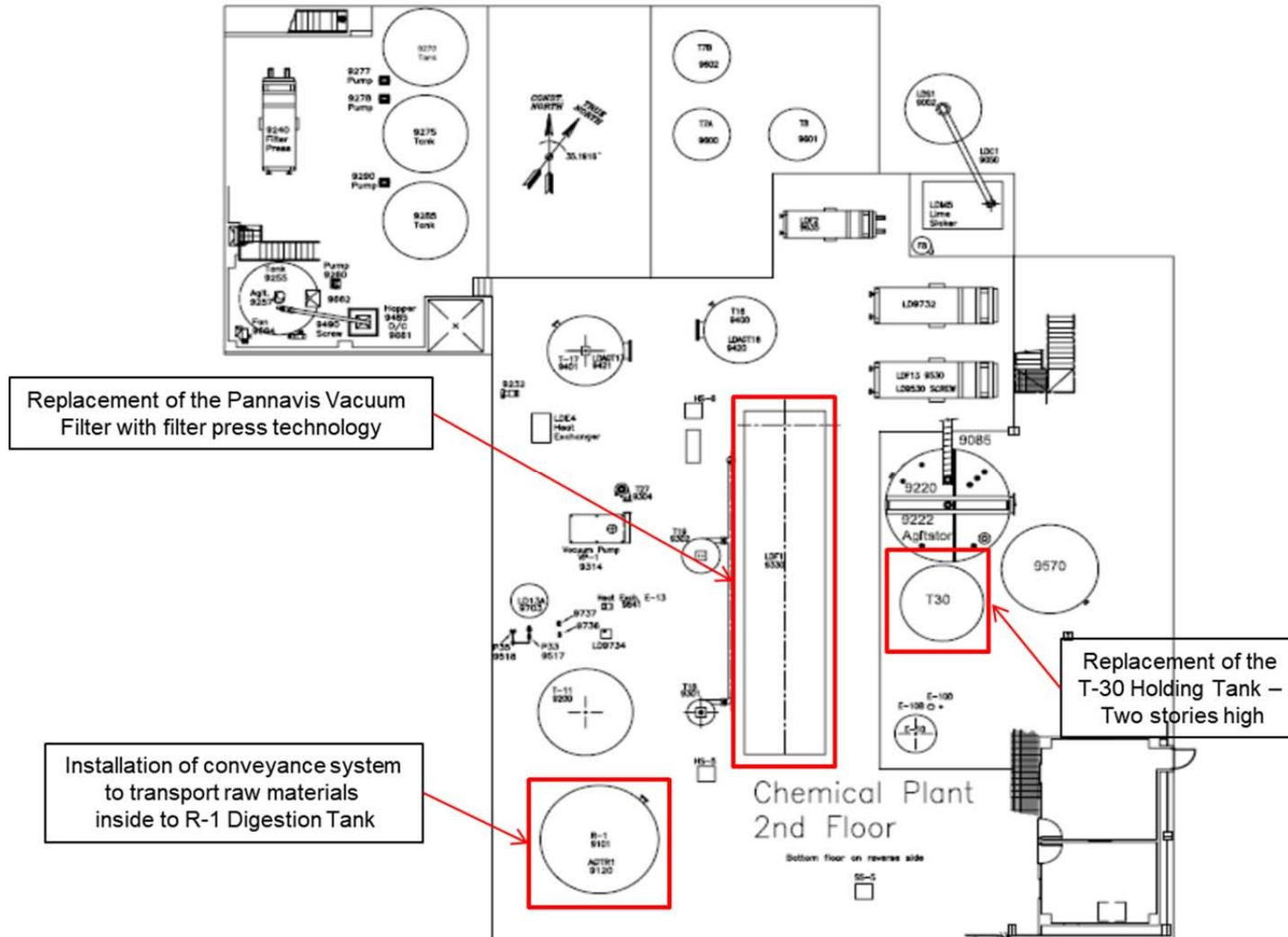
**Figure 3-3** Proposed alterations to the CPF second floor.
