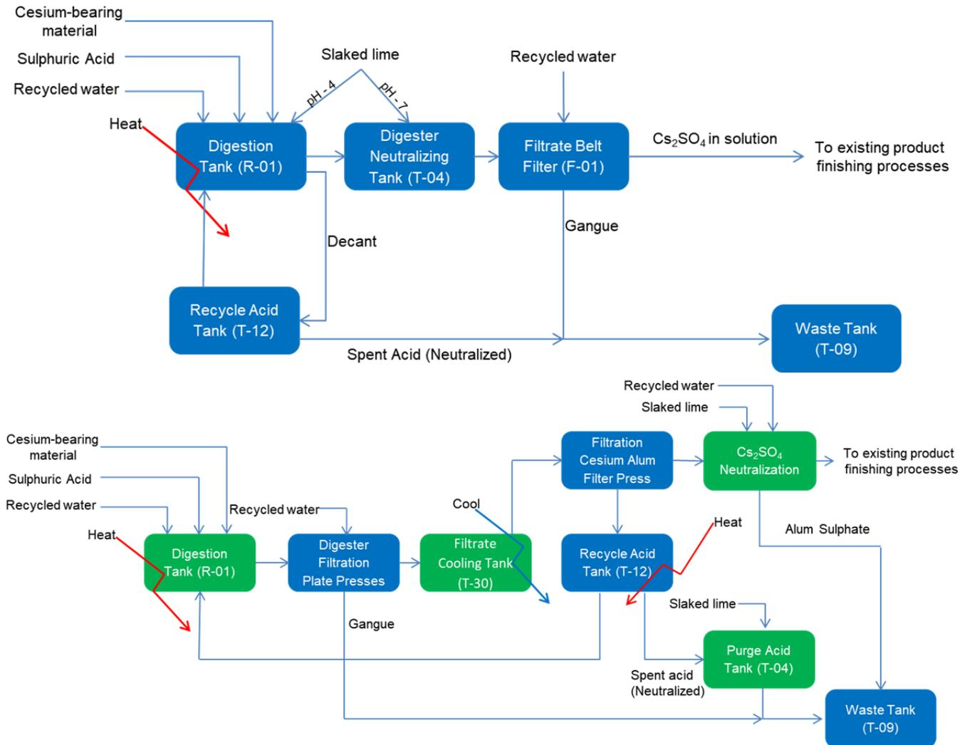
**Figure 3-4 CPF equipment and process current configuration (top panel) and proposed alterations (bottom panel) block flow process diagram. Green represents existing equipment and processes, while, blue indicates altered equipment and processes.**
