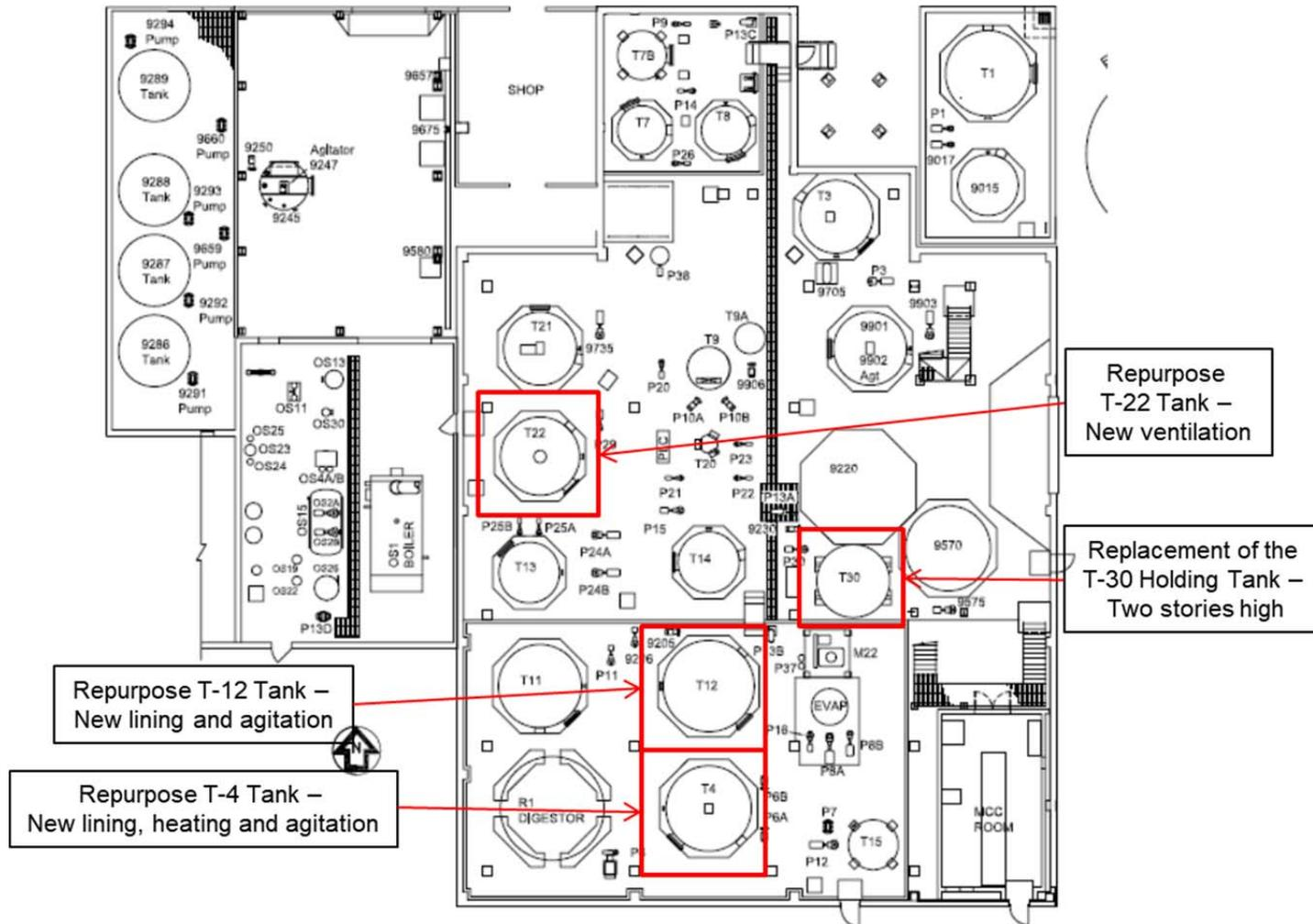
Figure 3-2 Proposed alterations to the CPF first floor.
