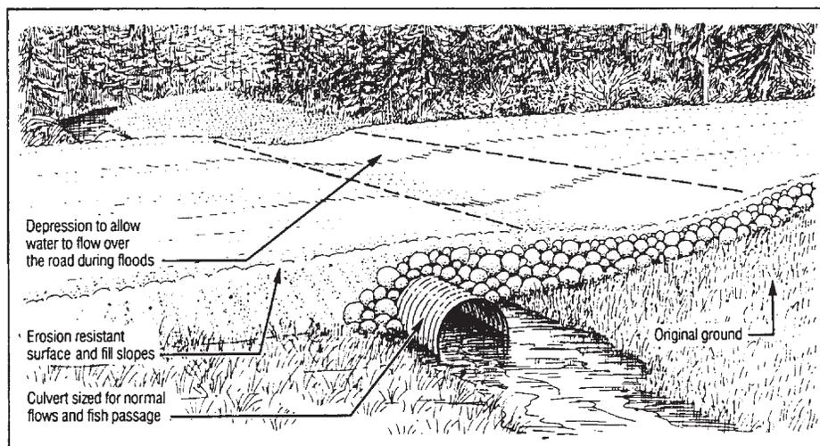
*Culvert with erosion protection and a depression to allow spillage over the road. Source: OMNR (1990).*
