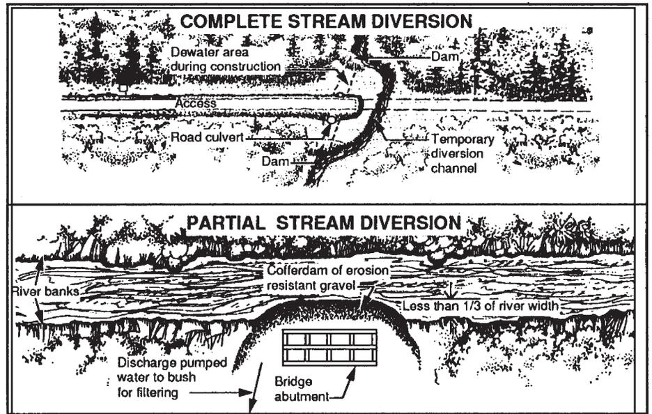
Stream diversion for dry crossing construction. Source: OMNR (1990).
