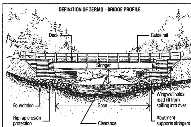
Components of a bridge. Source: OMNR (1990).
