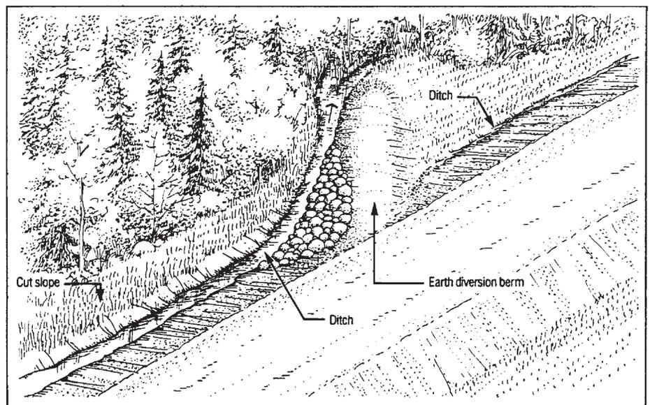
Forest floor filter - flow directed off right-of-way using a diversion berm.
