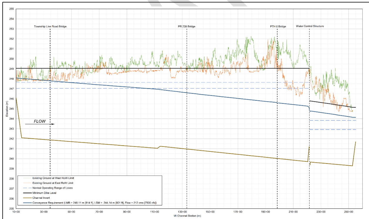
Figure 3: LMOC Water Surface Profile
