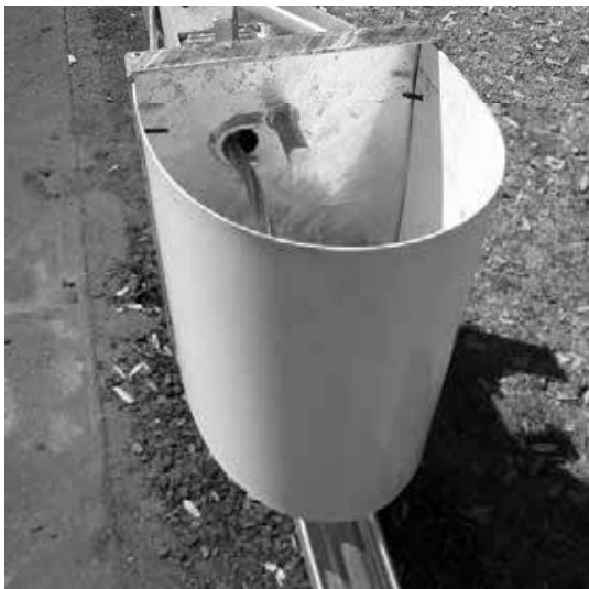
Figure 27. Attach nose using nylon push rivets.
