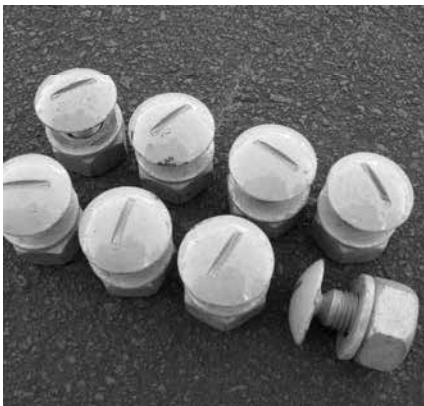
Shear Bolts 8 Required Roadside - 16 Median) K080123
