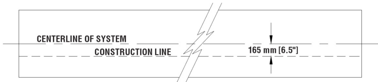
Figure 49 (Top view of concrete foundation)
