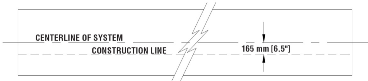
Figure 15 (Top view of concrete foundation)
