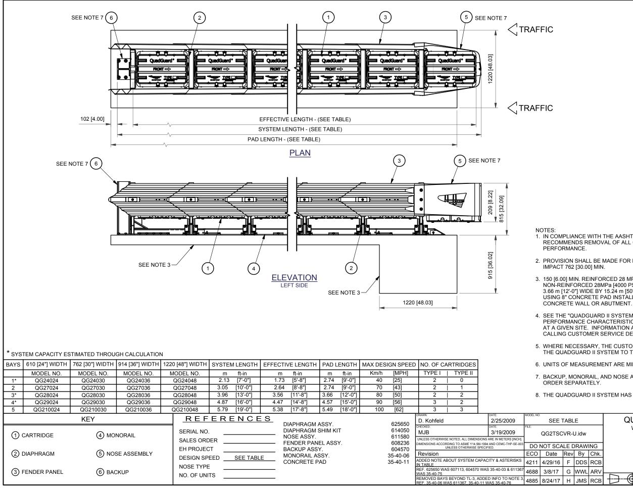
1. IN COMPLIANCE WITH THE AASHTO 2011 ROADSIDE DESIGN GUIDE, MANUFACTURER RECOMMENDS REMOVAL OF ALL CURBS AND ISLANDS TO ENSURE PROPER IMPACT
