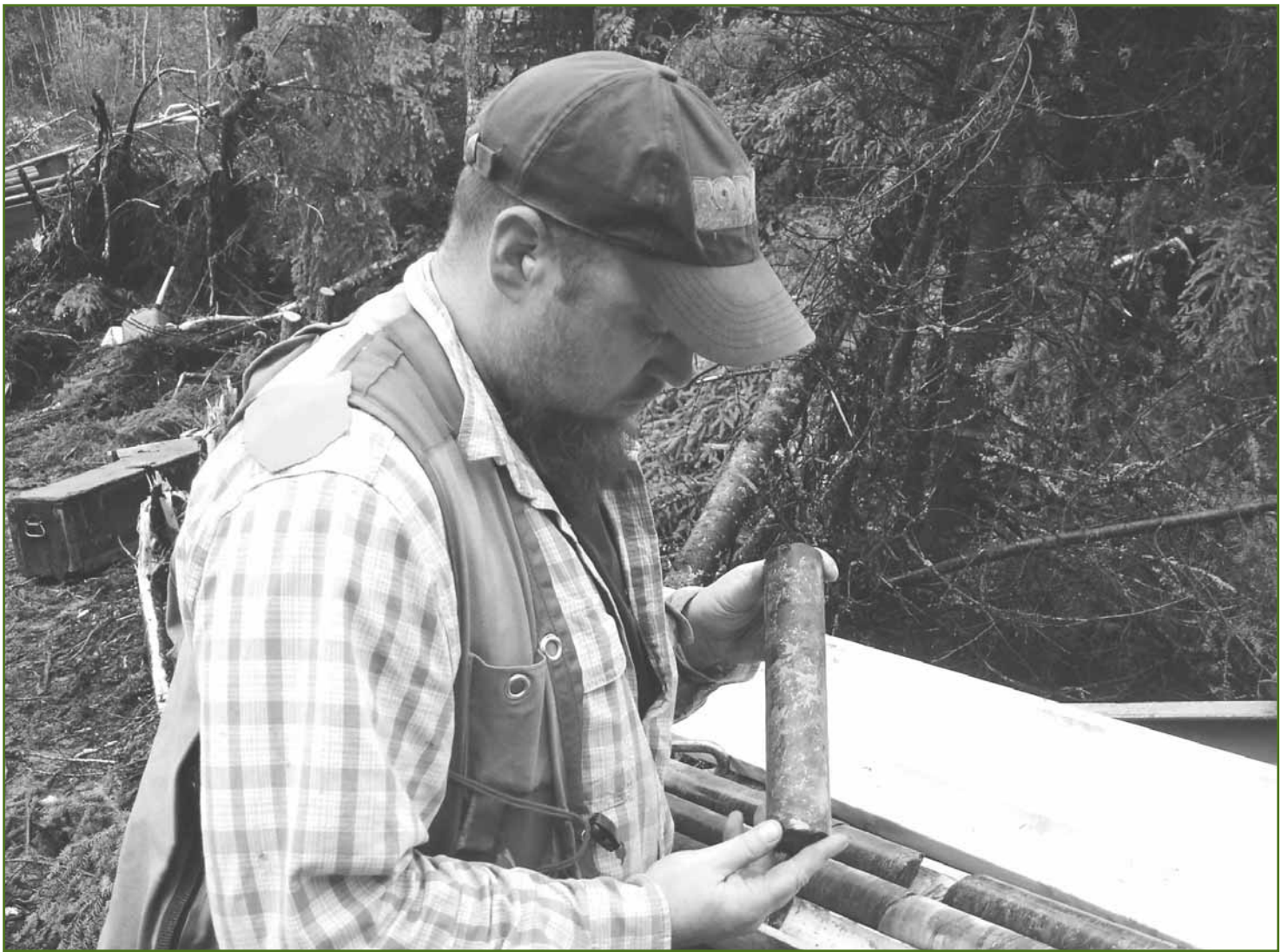
A mining survey worker examines a drill core sample for trace minerals. (Photo courtesy of Mustang Minerals).
