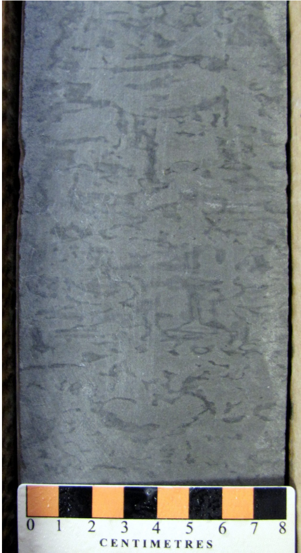
Figure 30: Core photographs of lithofacies unit 3–4 of the Middle Bakken Member in 7-3-12-29W1: a) bioturbated, very fine grained sandstone of lithofacies unit 3 at 814.5 m; b) mottled, very fine grained sandstone of lithofacies unit 4 at 813.3 m, showing the Nereites missouriensis trace fossils that are common in this unit; and c) rare thin coquina bed at 814.6 m.
