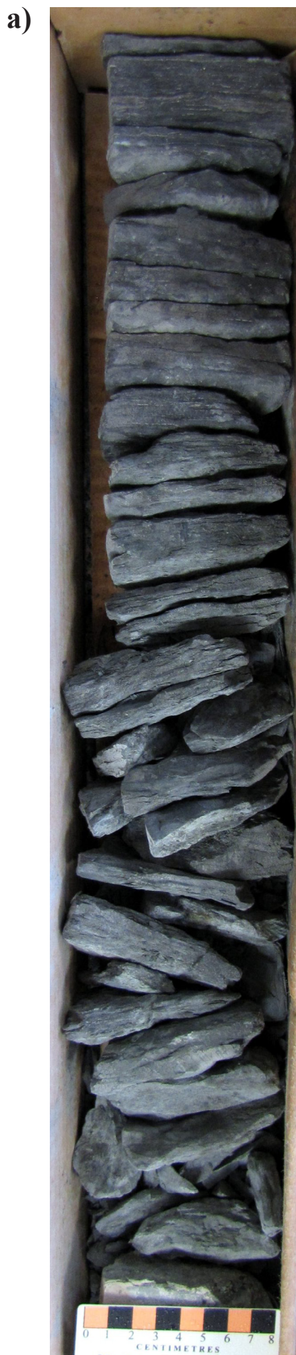
Figure 26: Core photographs of the Lower Bakken Member in 3-30-11-29W1: a) entire section from 864.3 to 865.3 m, b) close-up at a depth of 864.3 m.
