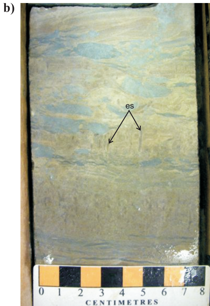
Figure 17: Core photographs of a) subunit 2c at a depth of 1003 m in 2-8-8-29W1, and b) escape structures (es) in subunit 2c at a depth of 1016.6 m in 4-28-7-29W1.
