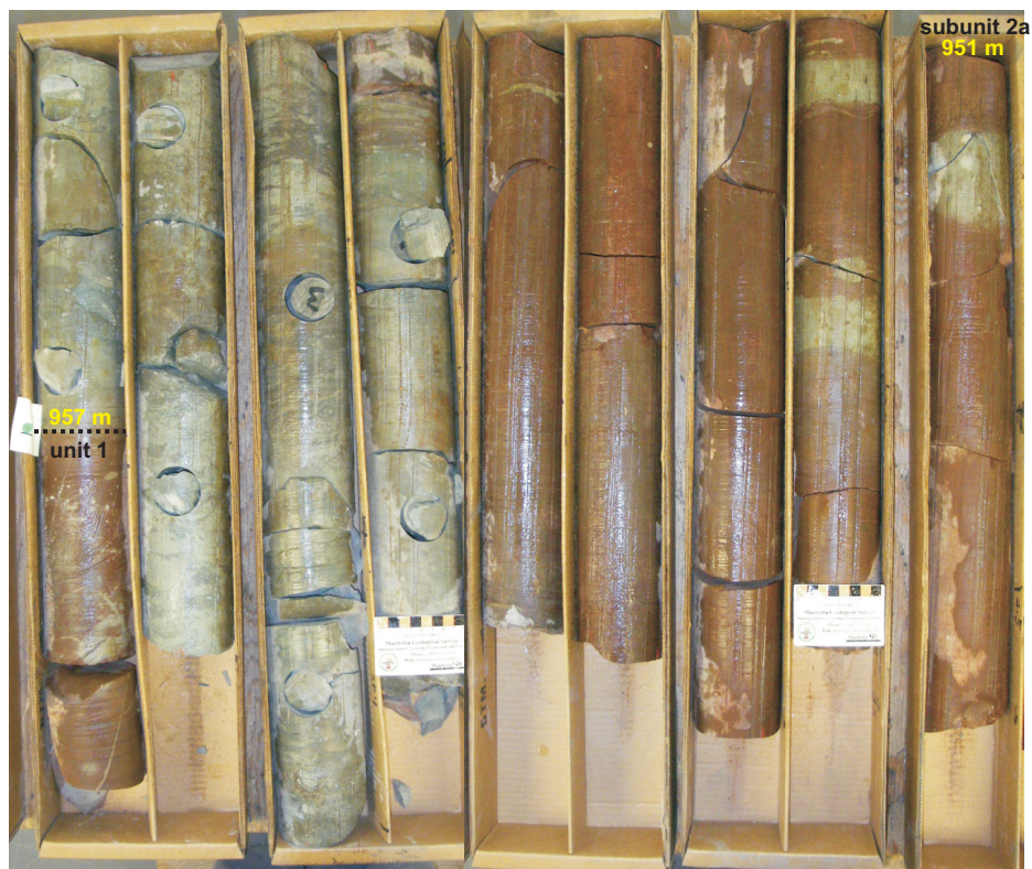
Figure 15: Core photograph of subunit 2a at depths of 951 m (top left) to 957 m (bottom right) in 8-14-8-29W1, showing sections affected by oxidation and reduction.
