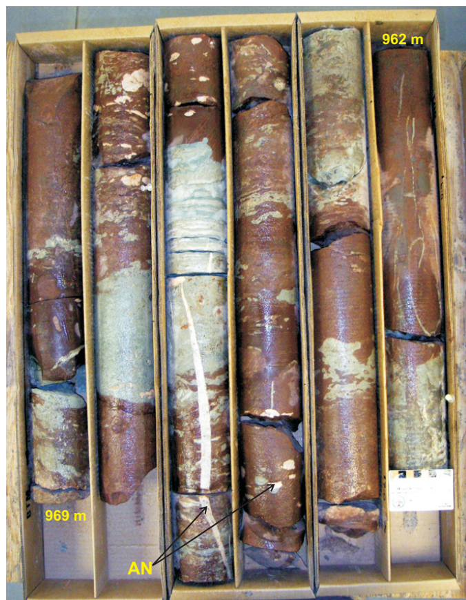
Figure 13: Core photograph of subunit 1b at depths of 962 m (top left) to 969 m (bottom right) in 8-14-8-29W1; note the red-brown (oxidized) and light grey-green (reduced) redox haloes; nodules and veins are anhydrite (AN).
