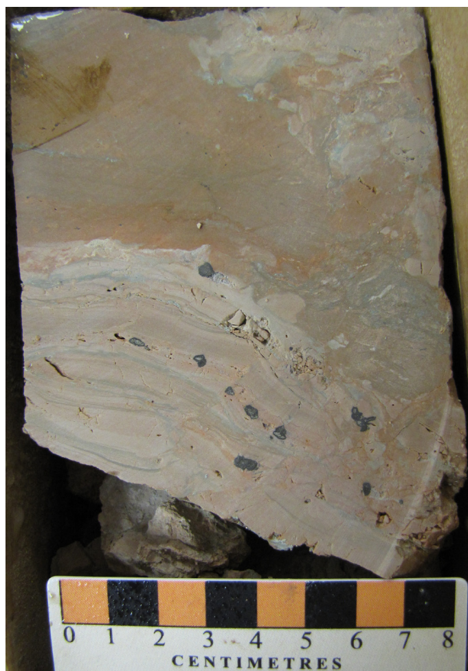
Figure 12: Core photographs of subunit 1a from 9-9-21-29W1, showing a) Birdbear-Torquay contact, and b) brecciated silty dolostone within silty shale matrix.
