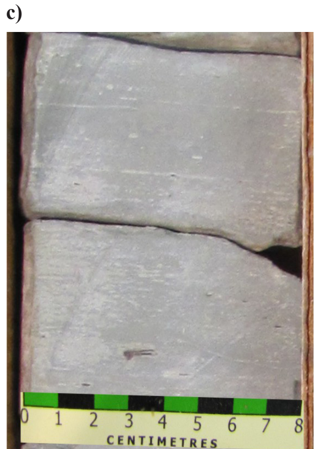
Figure 31: Core photographs of the Upper Bakken Member showing variegation: a) normal black shale, b) dark purple shale, and c) grey-green shale.
