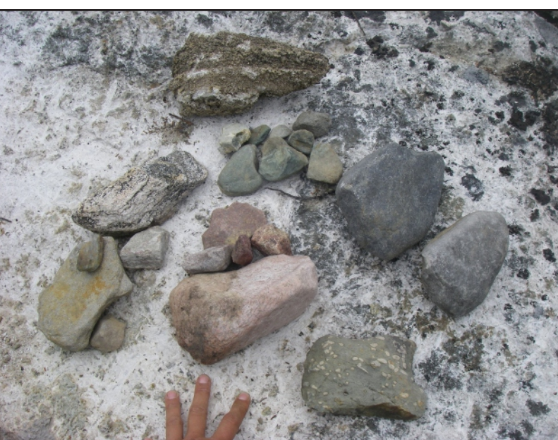
Various erratics collected at Pitchblende Ridge; used to help understand the location of source areas, and transport distance, for till at the site
