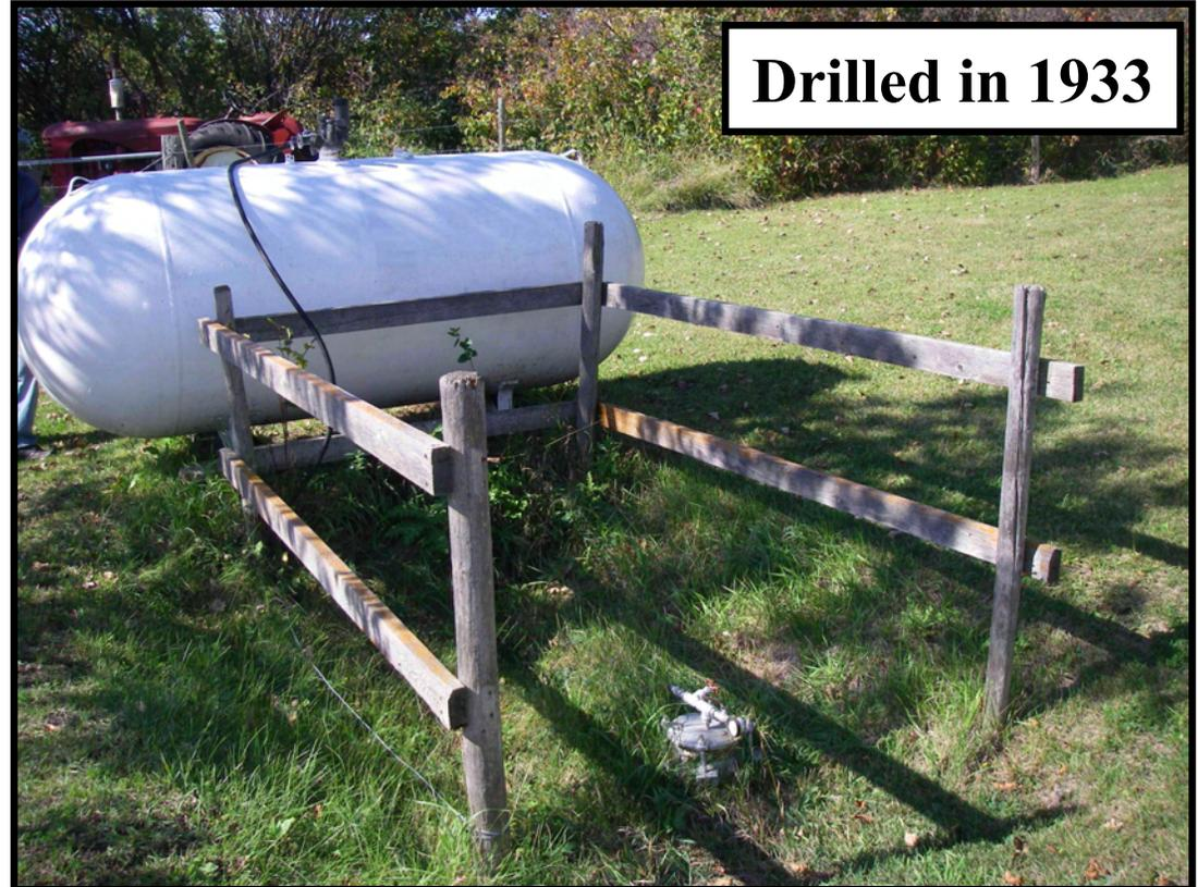
Two capped gas wells with pressures of  $\sim 276$  kPa, near Manitou, Manitoba.
