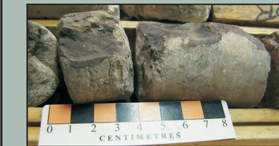
Figure 6: Oil staining in the Severn River Formation in the Houston Oils et al. Comeault Prov. No. 1 core.
