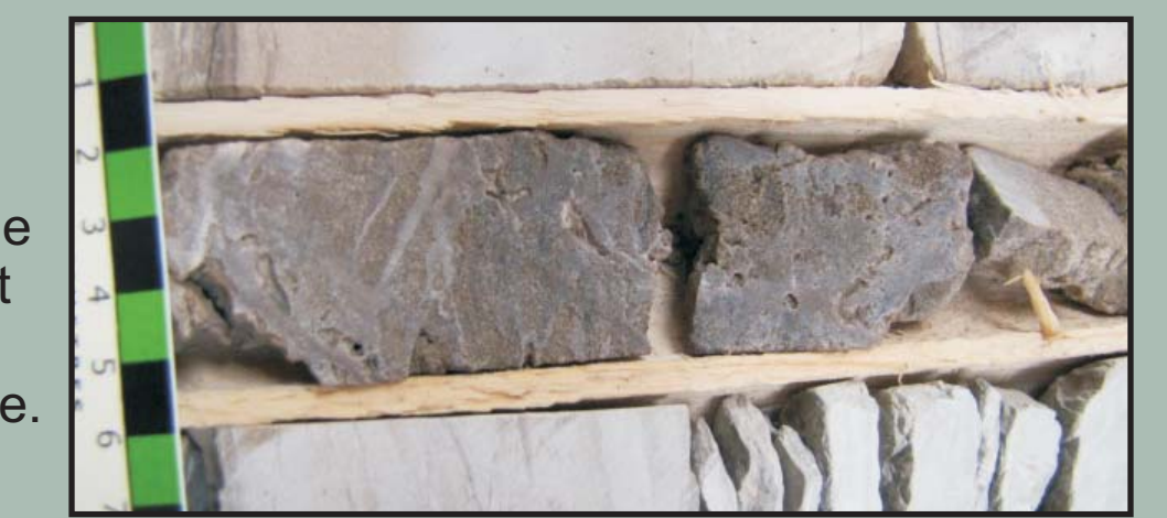
Figure 6: Oil staining in the Severn River Formation in the Houston Oils et al. Comeault Prov. No. 1 core.
