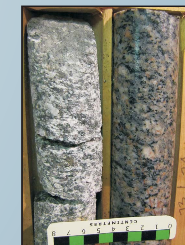
Precambrian weathered and unweathered granite Manitoba Hydro Conawapa Axis DX Dx1000
