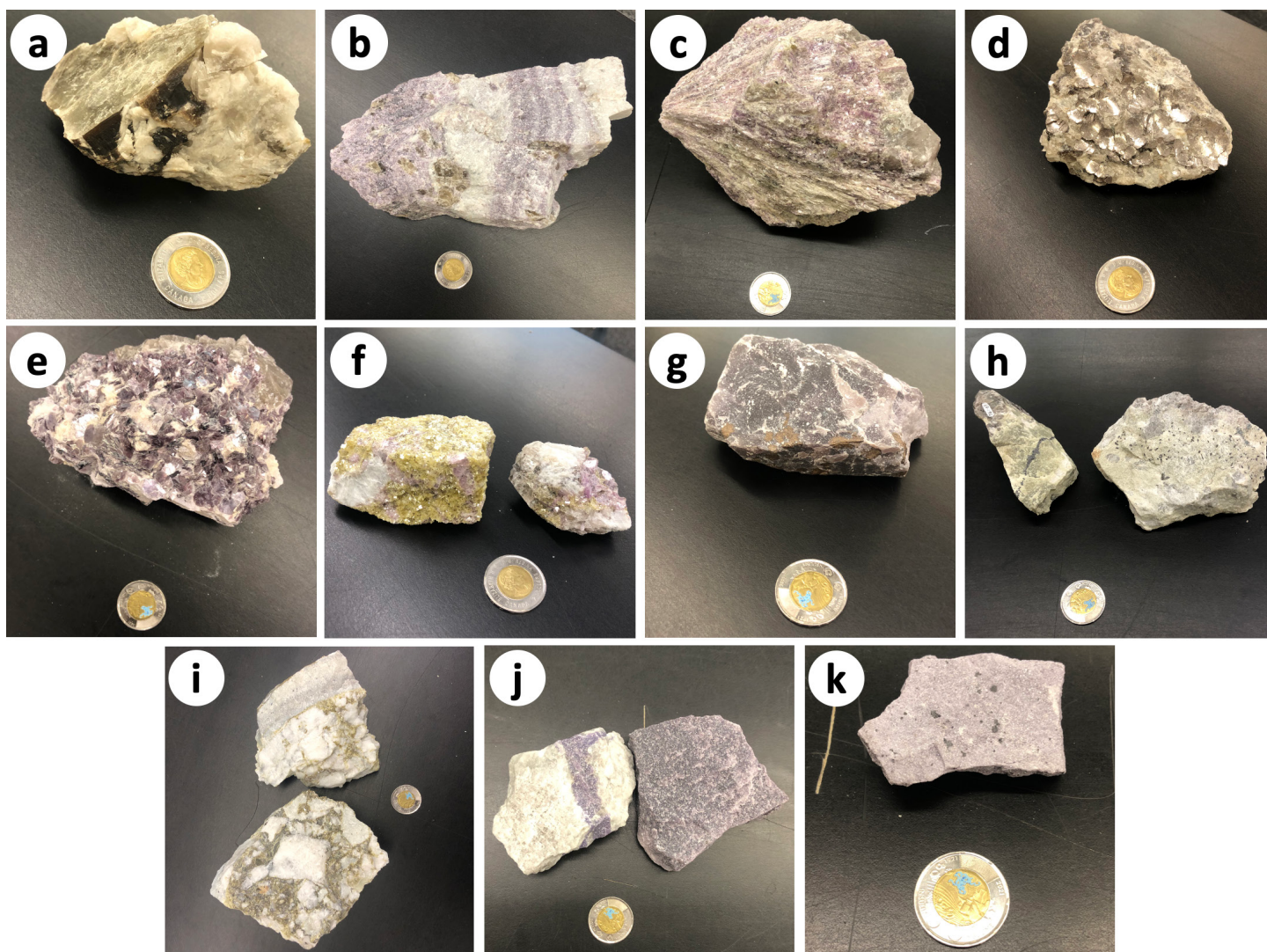
Figure GS2025-3-5: Assorted micas from the Tanco pegmatite of the Cat-Lake–Winnipeg River pegmatite field: a) pegmatitic muscovite (+albite) from zone 20; b) saccharoidal lepidolite (+aplitic albite, quartz) from zone 30, showing compositional banding; c) muscovite+Li-muscovite after rubellite (+quartz) from zone 40; d) coarse-grained ball-peen Li-muscovite (+quartz, albite) from zone 40; e) coarse-grained tabular lepidolite (+quartz, K-feldspar) from zone 40; f) coarse-grained late-stage green muscovite (+primary lepidolite, albite, quartz) from zone 50; g) massive saccharoidal grey muscovite from zone 50; h) saccharoidal pale green muscovite after microcline+quartz and wodginite (black specks) from zone 60; i) coarser grained green mica veining microcline and aplitic albite from zone 60; j) saccharoidal lepidolite veining in pollucite from zone 80; k) saccharoidal lepidolite (+Ta-oxides) from zone 90. Coin diameter is 3 centimetres.
