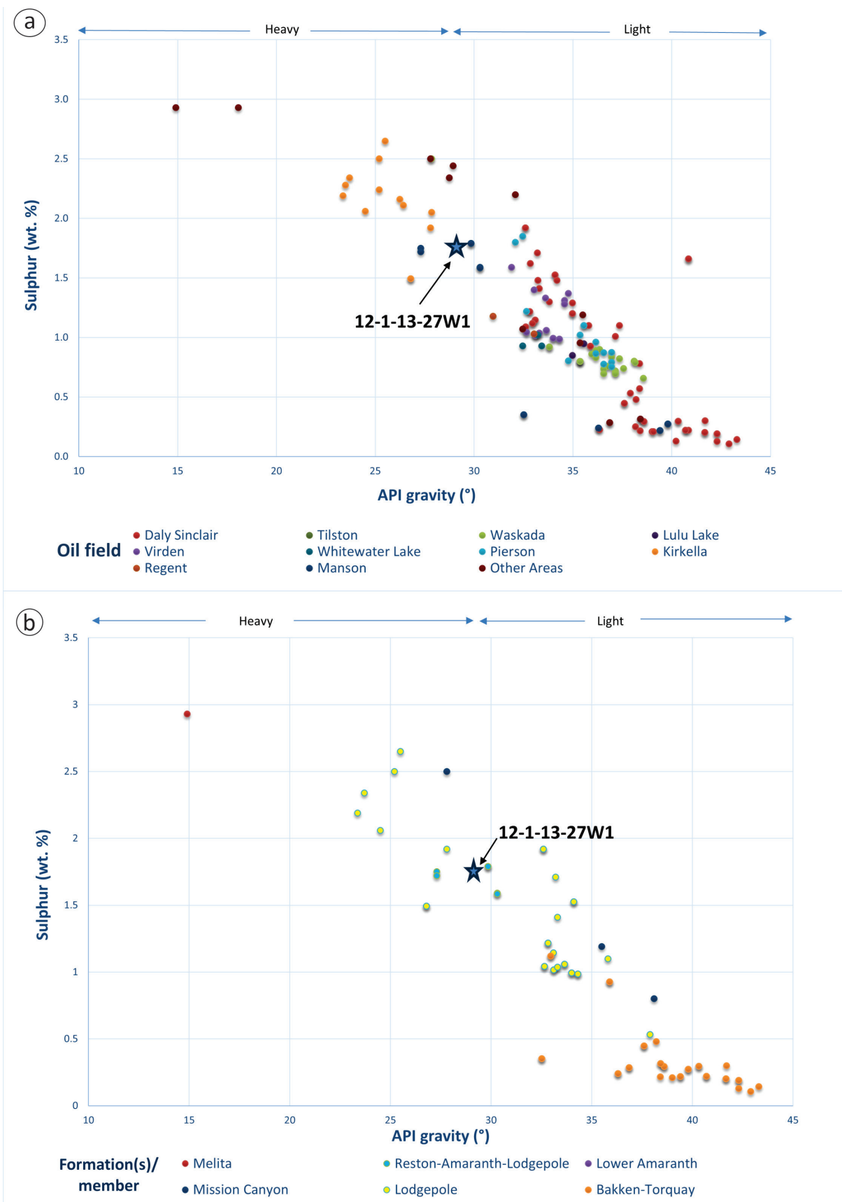
Figure GS2025-16-3: a) Chart of oil API gravity versus sulphur content by oil field; b) chart of oil API gravity versus sulphur content by producing formation(s)/member (Fulton-Regula, 2025; Manitoba Business, Mining, Trade and Job Creation, 2025b, c). Heavy high sulphur oil on the left and light low sulphur oil on the right. The oil sample from the well at L.S. 12, Sec. 1, Twp. 13, Rge. 27, W 1 st Mer. (abbreviated 12-1-13-27W1; oil and gas well licence 9990), southwestern Manitoba, is denoted by a star.
