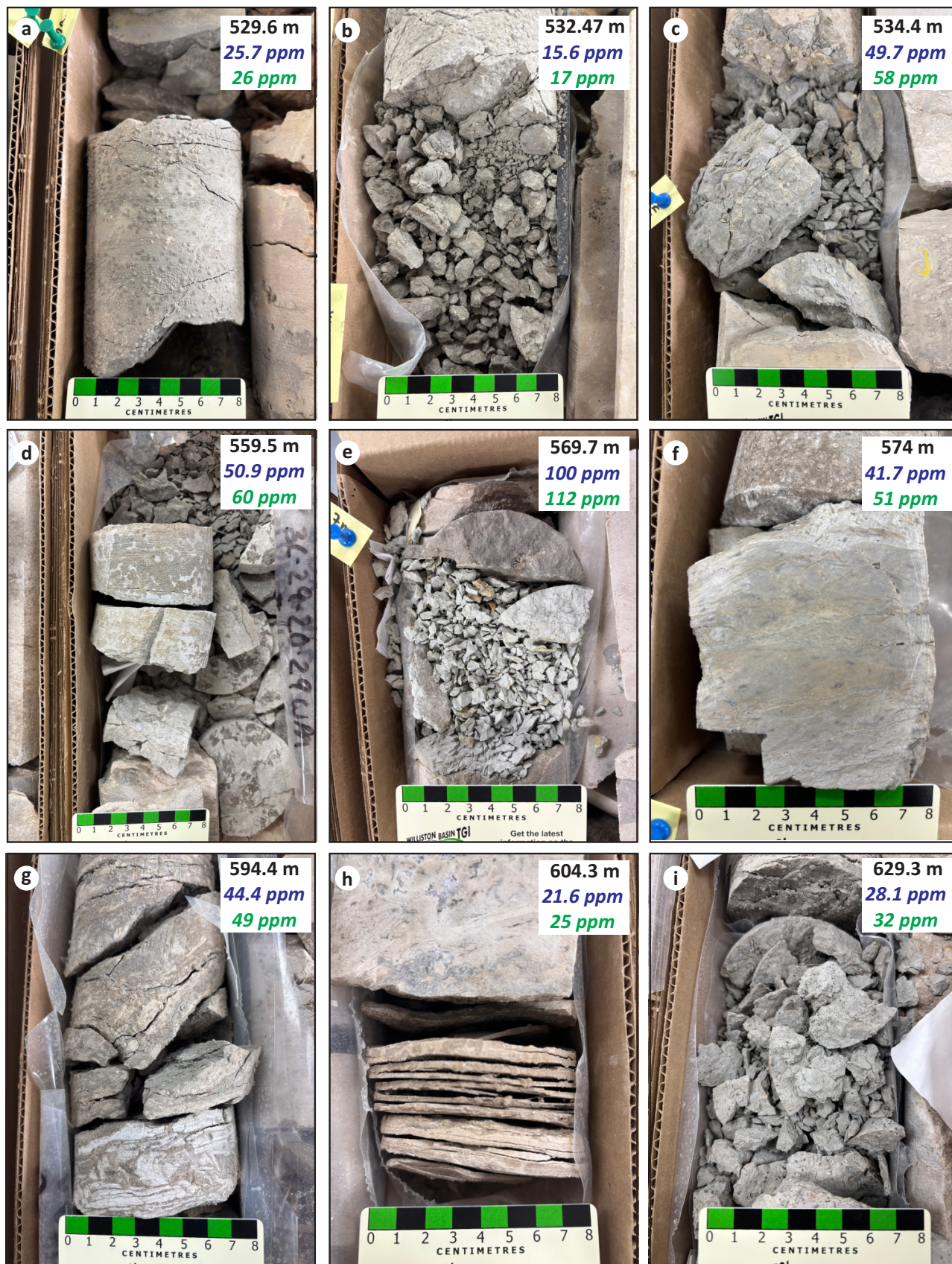
Figure GS2025-13-3: Photographs of the nine mudstone sampled sections in the Manitoba Potash Corporation (MPC) 3-29-20-29W1 core: a–c) Seward Member; d–e) upper Wymark Member; f–h) middle Wymark Member; i) lower Wymark Member. Note that the Saskatoon Member within the MPC core does not have any argillaceous, siliciclastic mudstone intervals, thus it was not sampled. See Figure GS2025-13-2 for sample locations along the core. Lithium concentration from each sample is shown in blue and green for four-acid and sodium peroxide fusion digestion methods, respectively. Samples are presented in stratigraphic ascending order (true vertical depth is shown in black).
