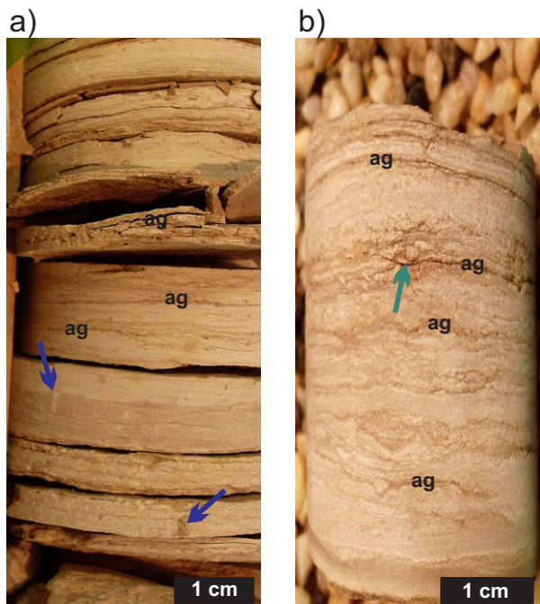
Figure GS-14-7: Core from the Merland et al. Whitebear Creek Prov. well showing examples of lithofacies I (laminated peloidal-skeletal mudstone to wackestone) from the intertidal lithofacies association: a) microbially laminated mudstone showing fissile, argillaceous laminae, with desiccation cracks (blue arrows), from a depth of 37.19 m; b) microbially laminated mudstone with thin bed of peloid-intraclast packstone (green arrow), from a depth of 36.24 m (modified from Ramdoyal, 2012). Top direction of core is top of image. Abbreviations: ag, argillaceous laminae.
