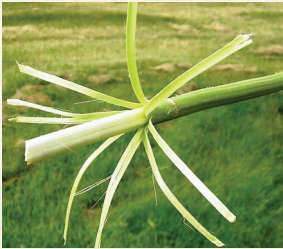
HEMP STALK WITH THE BARK (BAST FIBRE) PULLED BACK TO EXPOSE THE INNER CORE (HURD).
