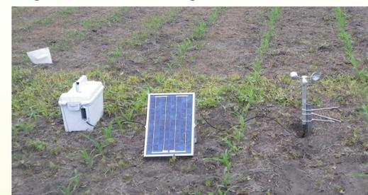
Figure 3. Solar powered data recorder and anemometer.
