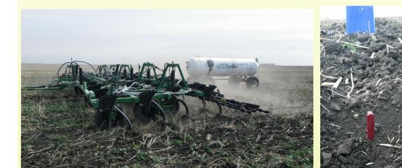
Figure 6. NH<sub>3</sub> application to dry soil and injection depth.
