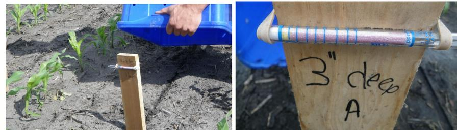
Figure 1. Installing chamber and reading the dositube.
