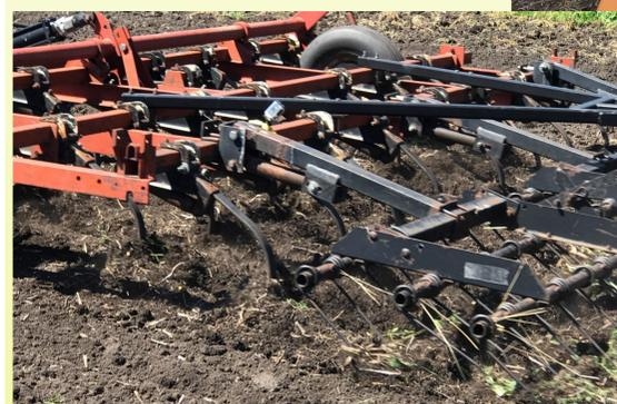
Figure 2: Operating field cultivator up and down slope.
