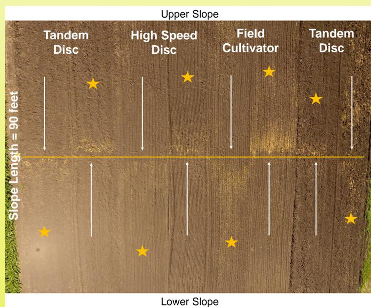
Figure 3: Aerial photograph of corn kernel distribution after tillage. Orange stars indicate farthest kernel found from the original trench line (orange centre line). White arrows indicate direction of tillage.
