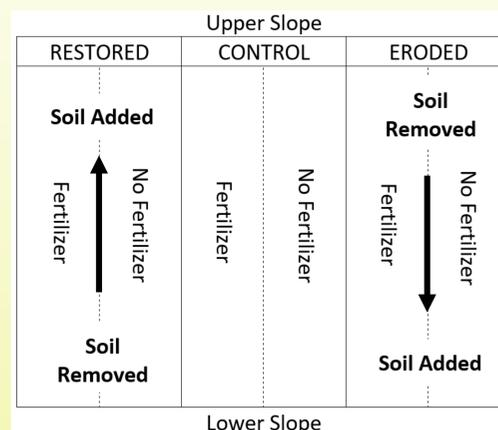
Figure 5: Layout of simulated erosion and restoration. For the “eroded” plot soil was removed from the upper slope and deposited at lower to simulate years of tillage erosion. For the “restored” plot, soil was removed from the lower slope and placed on the upper slope to simulate soil-landscape restoration.
