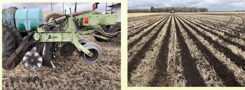
Figure 1-2. Strip till application of nutrients prior to seeding in 10" wide bands on 30" row spacing.
