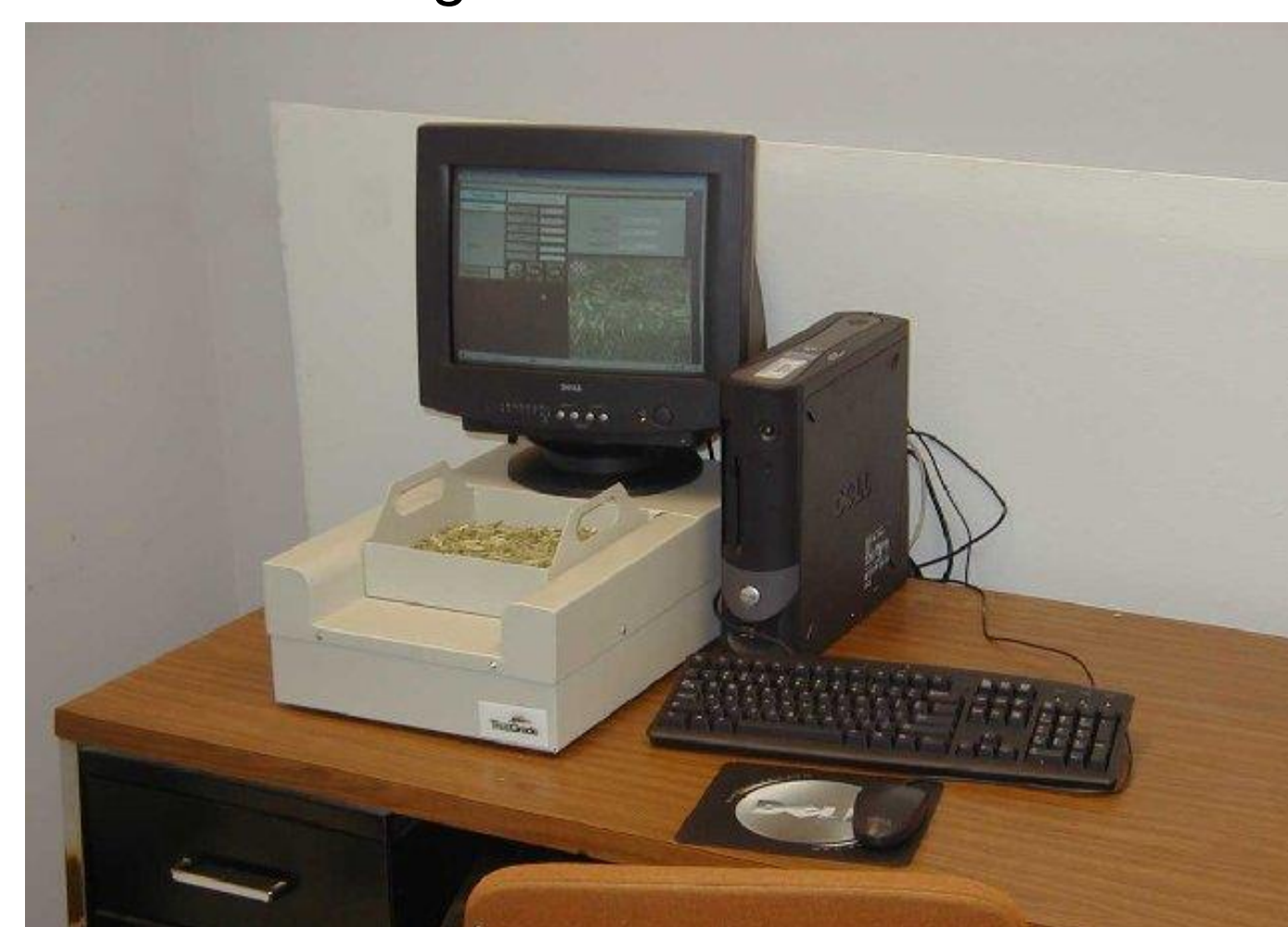
Figure 3. Determination of grade using Truegrade Hayscan (the higher the number, the better the grade).
