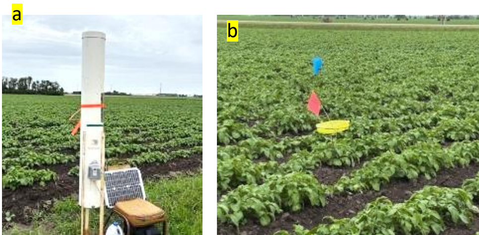
Fig. 9 a, b: Aphid monitoring is done using a suction trap and two yellow pans to trap aphids in or near the seed field.
