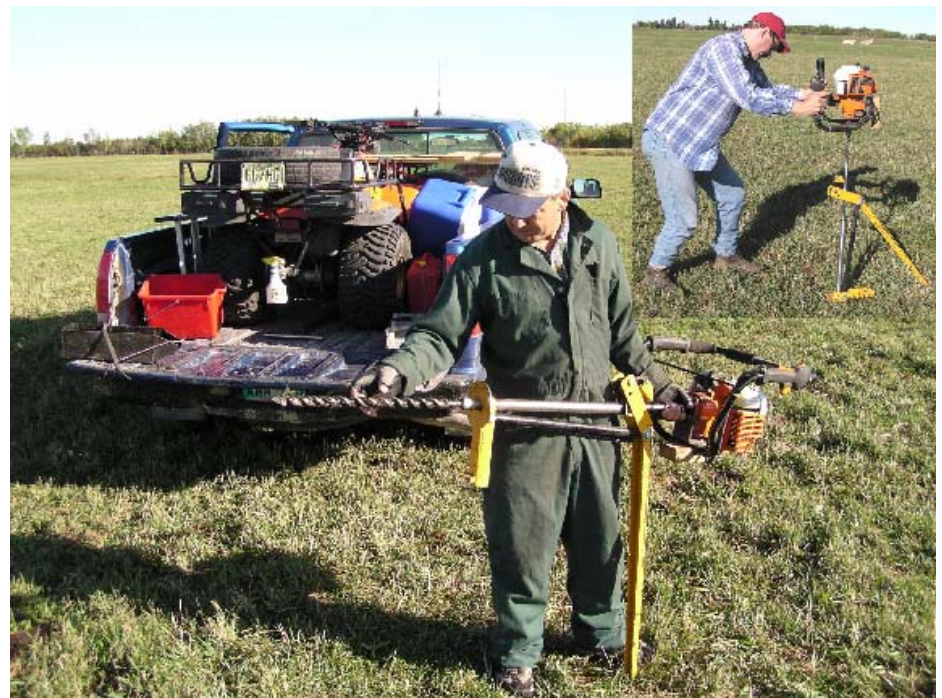
Figure 2. TSS Soil Sampler – a powered screw auger with a jacking handle for recovery of soil samples (available from aasoils.com ).
