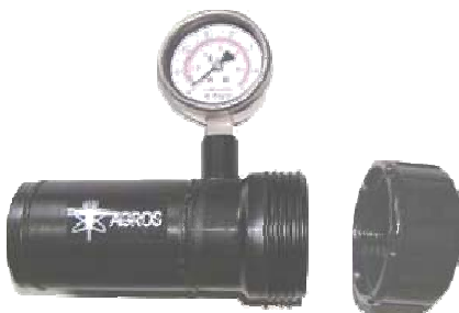
Figure 5. Ammonia test meter included in the Nova meter model Mk3 field test kit (available from www.agros.se ).
